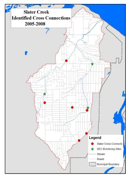
Figure 7 Slater Creek Cross Connections
