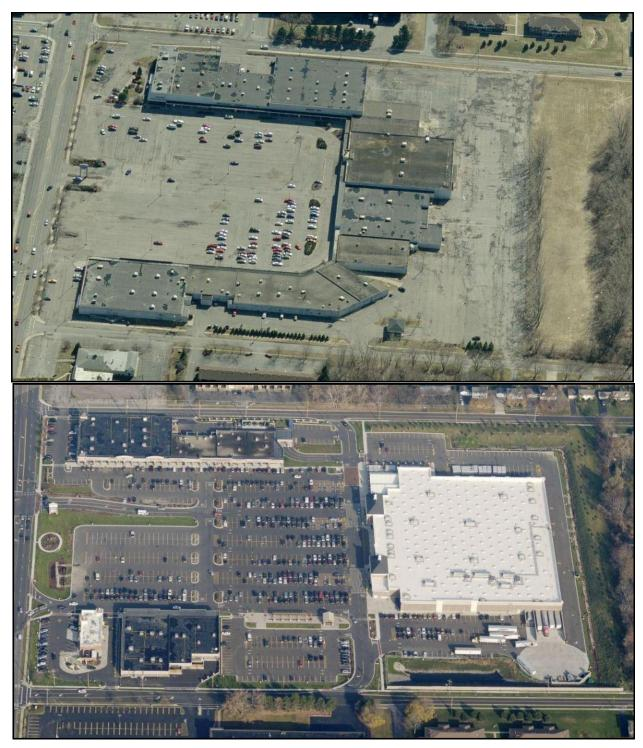
Figure 13 Northgate Plaza in 2009 (above) and 2012 (below) Showing impervious area reduction and increased green space
