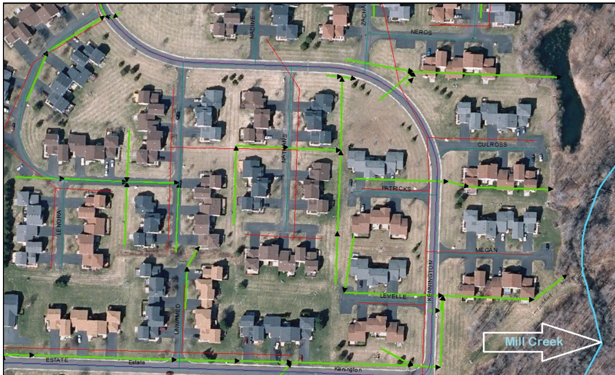
Figure 8. Potential Retrofits include GI in green space at this dense multi-family residential development from the 1970's that lacks stormwater treatment.
